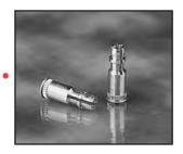
CFKSSB spring-top standoffs are designed for permanent installation into PC boards by pressing into a drilled or punched hole. The spring-action post provides quick attachment and removal of PC boards, with a simple snap eliminating the problems associated with loose hardware.
